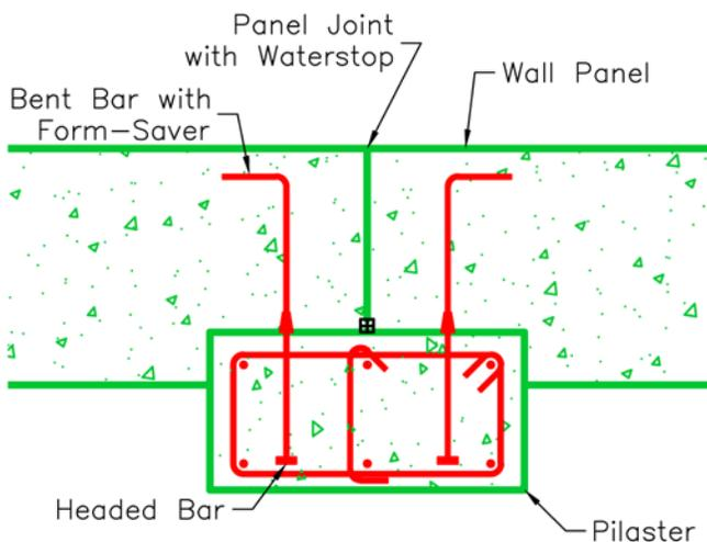
*Fig. 11 - Pilaster (plan view)*
