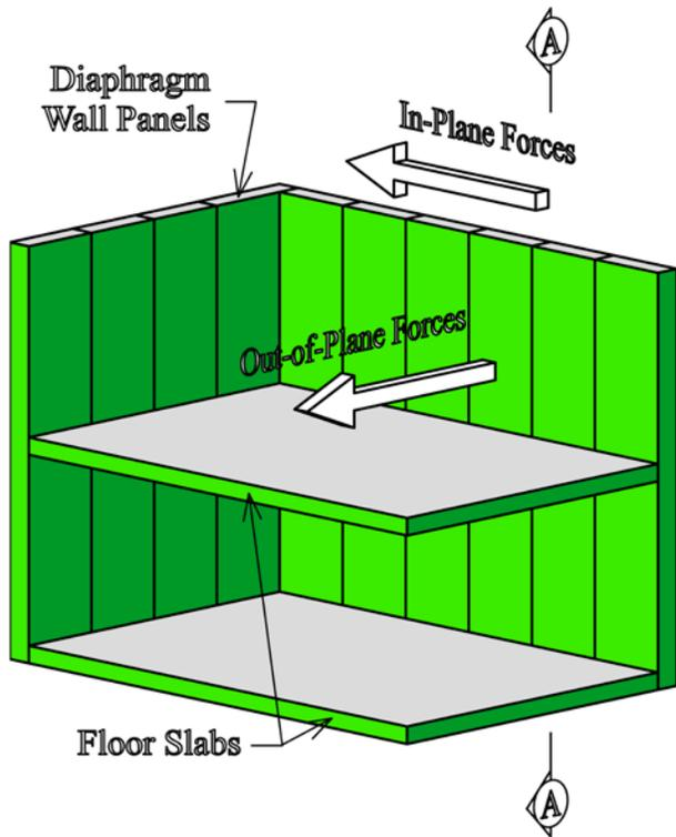
*Fig. 1 - Forces Acting on Diaphragm Walls
