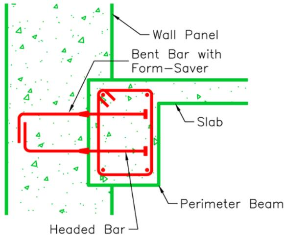
*Fig. 10 - Perimeter Beam (cross-section)*
