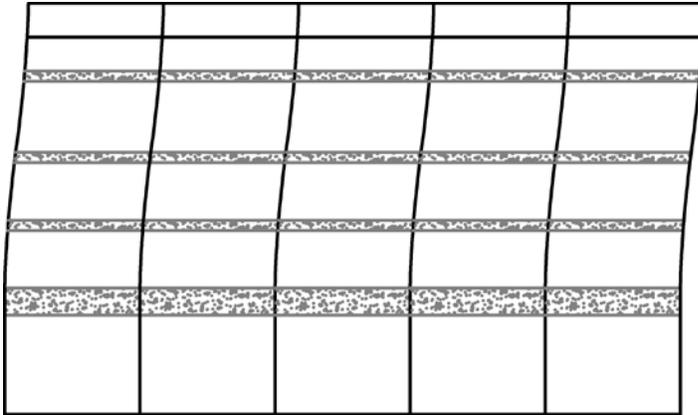
Fig. 8c - In-Plane Deformation (full restraint)
