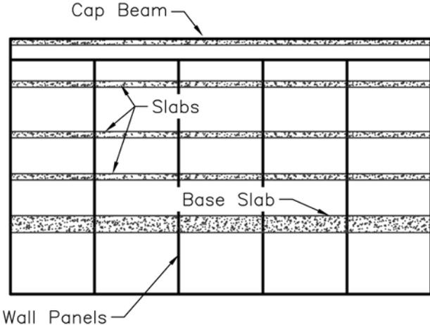
Fig. 3 - Wall Elevation
