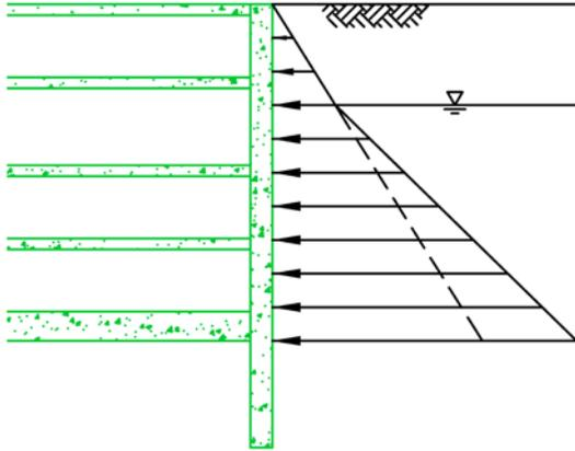
Fig. 2 - Earth Pressures (Section A-A from Fig. 1)
