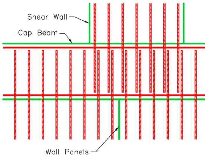
Fig. 9 - Shear Wall Connection (Elevation View)
